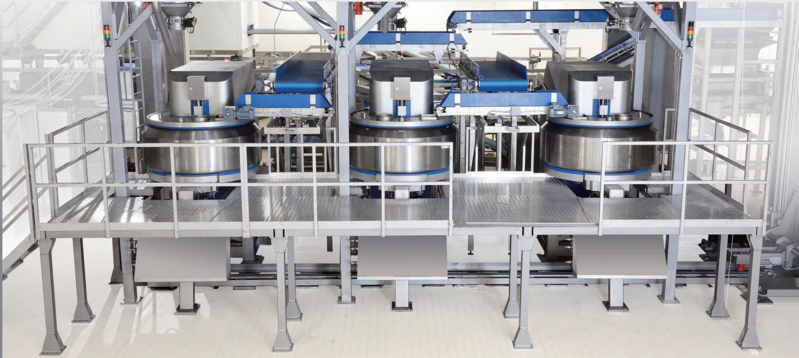
Spiral mixing machine with a bowl cooling system
